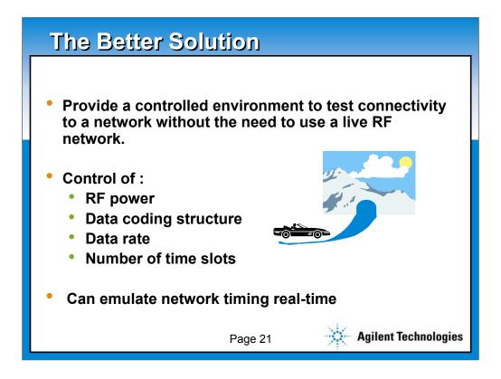
Our solutions provide a network on a bench. It's a matter of setting several IP addresses correctly. Our products provide easy control of the coding structure and associated data rate, the RF power level, added noise in CDMA systems, and the ability to monitor the messages.
