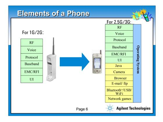
One segmentation of device functions are shown on the left, in green. These same functions still exist in newer designs, but have been augmented by additional features.
