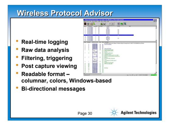
Here is an example of a protocol log on WPA. The upper window is the sequence of messages, while the lower window provides the details of the message in blue in the upper window.
