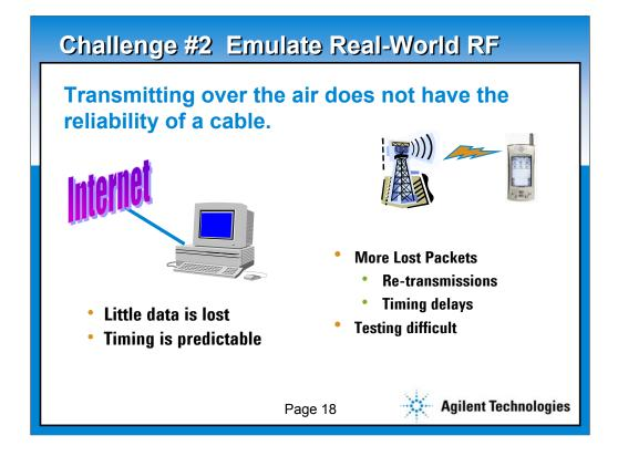
The environment of a packet connection that uses a radio link is very different than one that is wired. While the protocol for each system allow for lost packets and the control functions that result in a re-transmission, the occurrence on the wired Internet is very low, while the link over-the-air typically targets an operating point near 1% lost packets.
