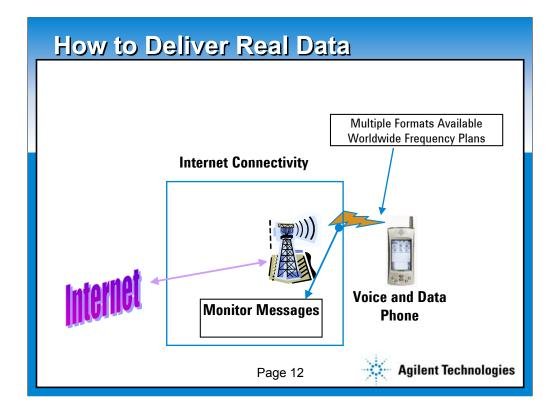
The wireless industry has multiple formats. The Internet is shared by all, however. What is needed is a transducer that can connect to the Internet with a network connection, and to the phone with a cabled connection that carries the properly formed RF signal of the format being tested. In the middle, a monitor of the messages needs customization for each format, as well.
