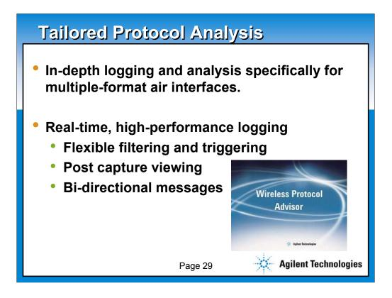
The Agilent Protocol Analysis is performed in a software package called the Wireless Protocol Advisor (WPA). This is a program that runs on a PC and connects to our base station emulators with a network connection. WPA is included with each Lab application and Protocol Application.
