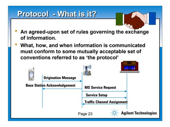
In its simplest form, Protocols are a list of rules on what can be said, and when between network entities. The phone can only talk to a base station, but the base station has two underlying networks, the circuit switched phone network, and the packet switched data network, commonly called the Internet.
