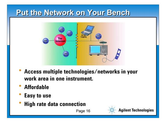
An improved solution is to put wireless access on your bench. The test products become the transducer between the Internet and the wireless device being developed or tested. Full message instrumentation is available for the link.
