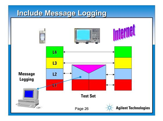
Along with the actual connection to the Internet, there is the ability to log messages carried in both directions on the RF link.
